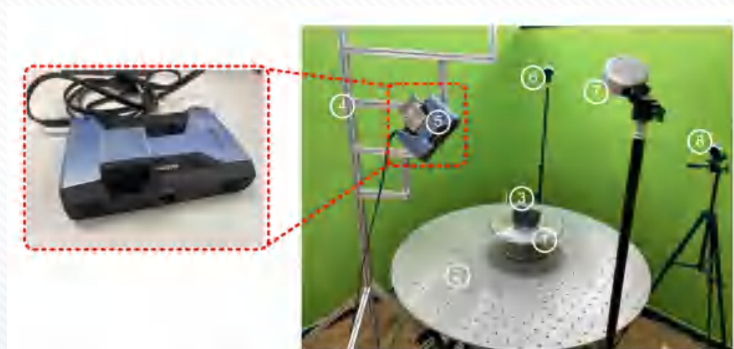
Figure 3. The task-specific model acquisition equipment. (a) 1 is a Rotating turntable for objects with multiple scales. 2 is a tracking marker. 3 is a light-absorbing item. 4 is a lift bracket. 5 is the Shining 3D scanner. 6-8 are the realsense L515 cameras for capturing multiviews of objects.
